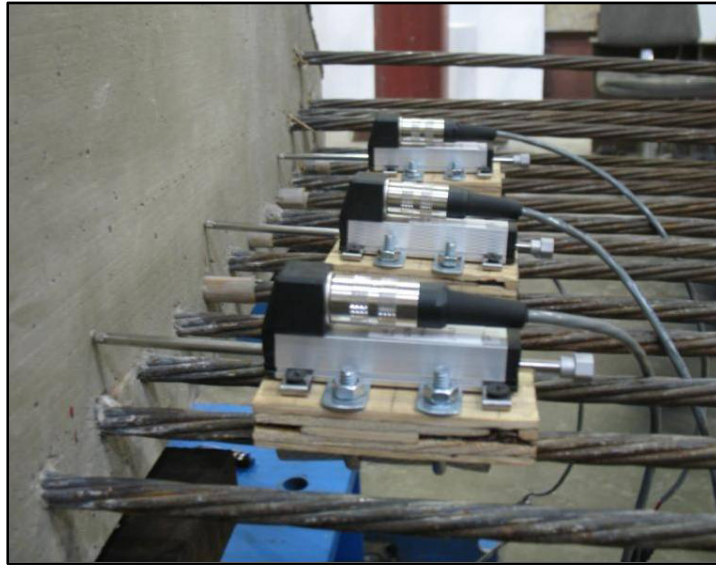
Figure 3-24 Linear potentiometers installed to measure strand slip.
